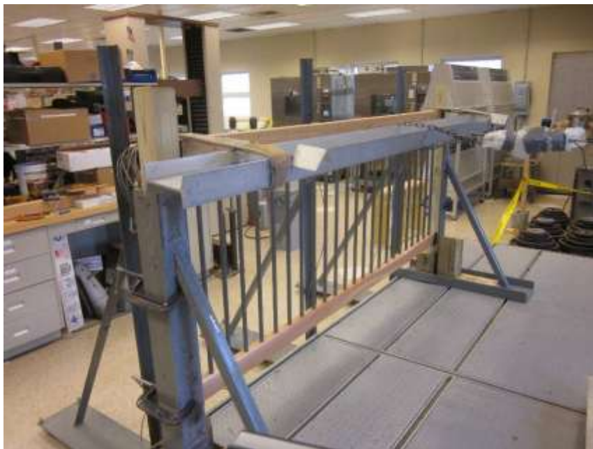
Photo No. 4 Concentrated Load at Both Ends of Top Rail (Brackets)
