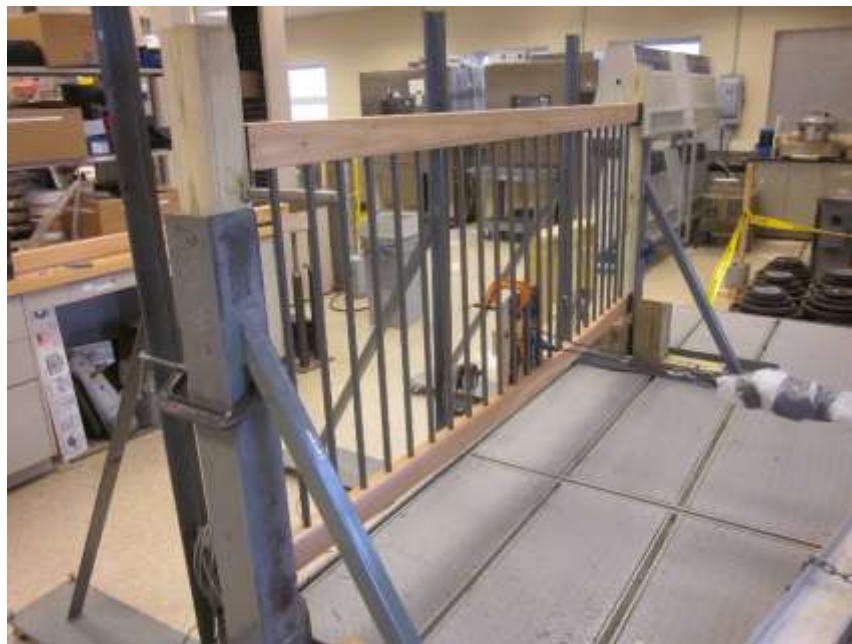
Photo No. 2 In-Fill Load at Bottom of Three Balusters
