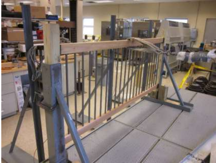
Photo No. 3 Concentrated Load at Midspan of Top Rail
