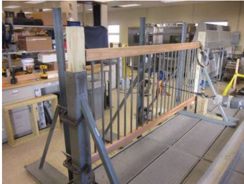
Photo No. 1 In-Fill Load at Center of Three Balusters
