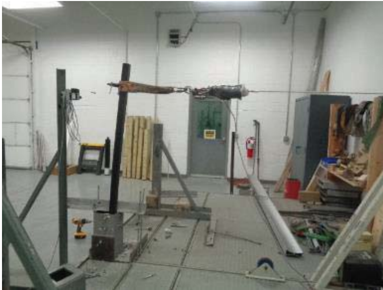
Photo No. 1 Concentrated Load Test on Inside Corner Bracket
