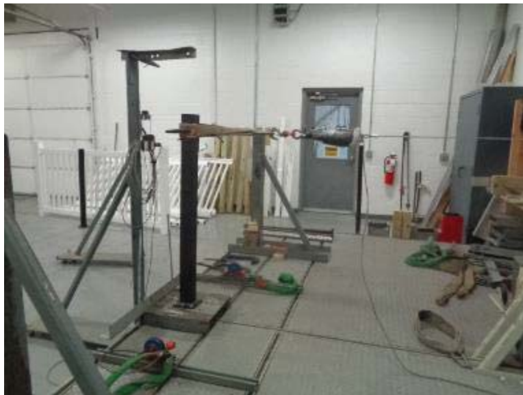
Photo No. 6 Concentrated Load Test on Surface Mount Post
