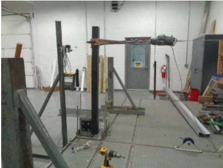
Photo No. 3 Concentrated Load Test on Outside Corner Bracket
