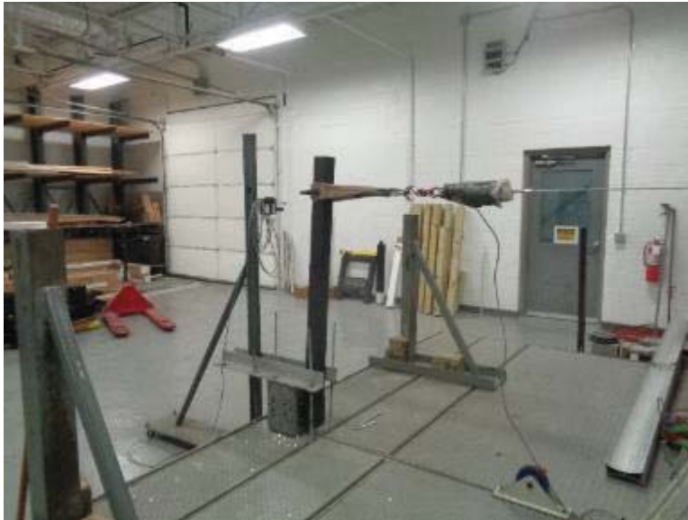
Photo No. 5 Concentrated Load Test on In-Line Bracket
